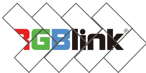
Example: 4K HDMI mapped over eight rotated displays connected to eight HDMI ARO™ outputs fitted to FLEXpro8. Preview connected sources via dedicated HDMI
