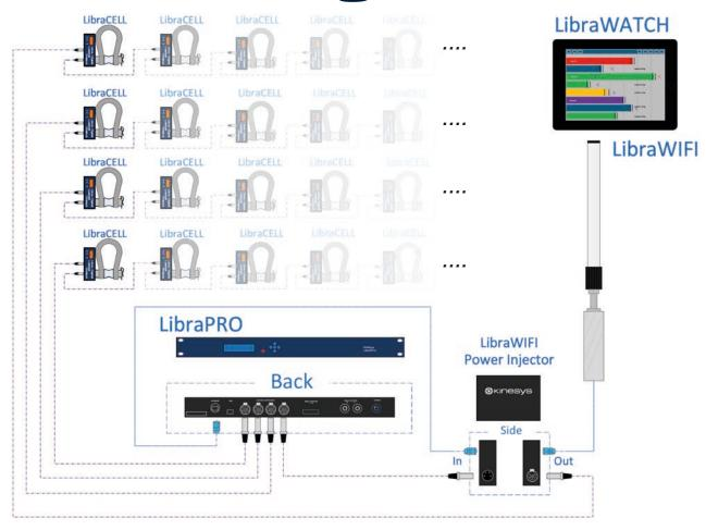
The diagram above shows the simple configuration of a Libra system. LibraPRO allows 25 LibraCELLs to be linked together on each of its four XLR4 outputs. LibraWIFI can be connected to LibraPRO's Ethernet port to permit the broadcasting of the data to portable devices. Libra is a simple, intuitive and extremely reliable load monitoring system.
